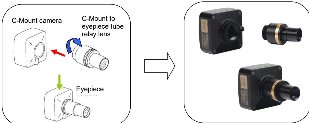
**STEP 3:** Attach (Insert) the eyepiece camera into the ocular tube or eyepiece tube
