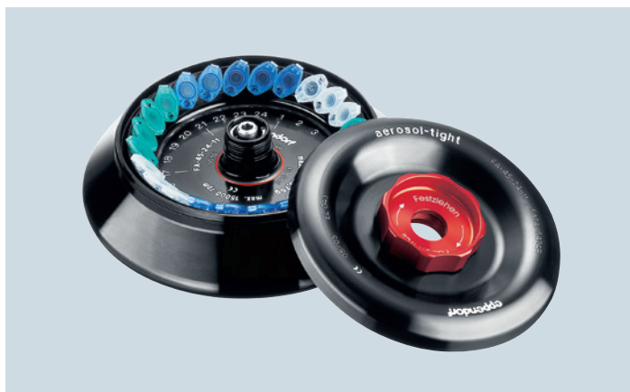
Aerosol-tight rotor for 24 × 1.5/2.0 mL tubes provides speed up to 21,130 × g /15,000 rpm. (FA-45-24-11; Order no. 5424 702.007).
